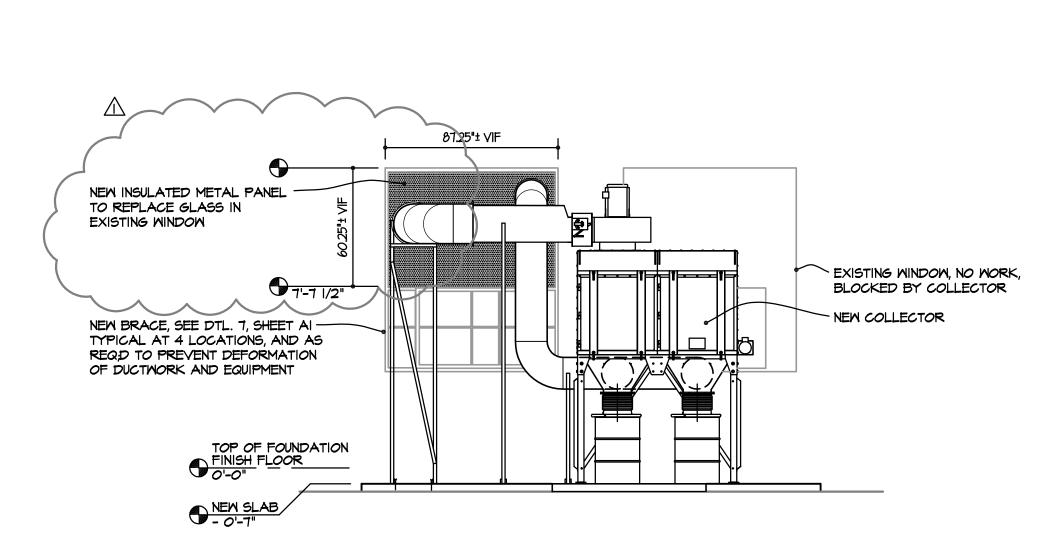
1 DUCTWORK LAYOUT ELEVATION
