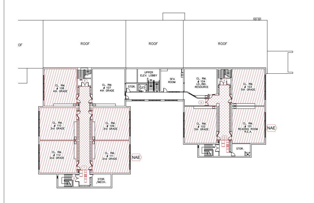
**\ASBESTOS ABATEMENT** SECOND FLOOR PLAN
