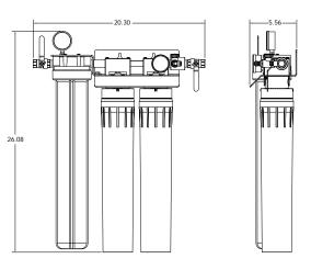
Note: Allow 3" of clearance at bottom of system for removal of filter bowls for filter cartridge replacement
