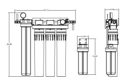
Note: Allow 3" of clearance at bottom of system for removal of filter bowls for filter cartridge replacement
