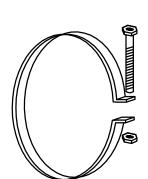
1' WIDE, 0.109" THICK STRAP WITH STANDARD ½"x6" BAND BOLT AND NUT.
